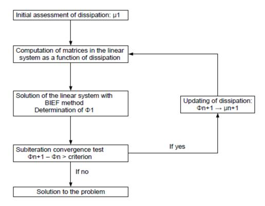
It seems that the most suitable iterative resolver for the linear system being considered is the direct solveur. That resolver is taken by default by the model. The matrix may previously be diagonally preconditioned. The user, however, may freely choose any other resolver and any other preconditioning as proposed through keywords in BIEF (see in § 8).
