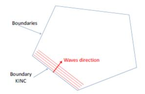
Example 2: Incident wave not normal to the boundary, constant bathymetry
